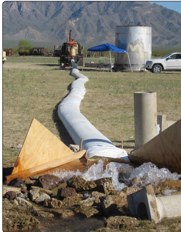
Groundwater discharge from the Butler Valley Aquifer test.
