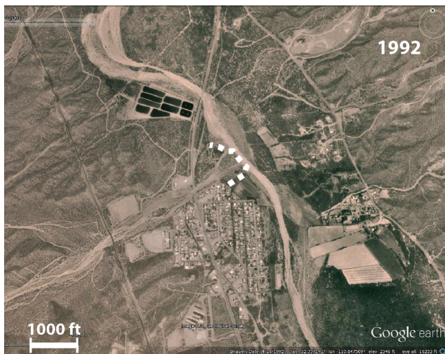
Figure 11. Sequence of aerial photos of the Tucson Wash – San Pedro River confluence illustrate the dynamic interaction between river floods and tributary floods. White dashed lines illustrate the approximate boundary between river and tributary deposits at each photo date. The large river flood of 1926 substantially eroded the Tucson Wash fan, which was still evident in 1935. By 1955, Tucson Wash alluvial fan had prograded over the former river channel. This trend has continued to the present, as the Tucson Wash fan has forced the river channel to the east and has covered most of the 1926 flood channel. North is up. Base imagery from the Soil Conservation Service (1935), Army Map Service (1955), Google Earth (1992), and National Agricultural Imagery Program (2103).
