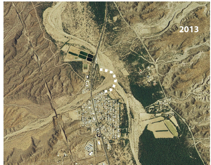
Figure 11. Sequence of aerial photos of the Tucson Wash – San Pedro River confluence illustrate the dynamic interaction between river floods and tributary floods. White dashed lines illustrate the approximate boundary between river and tributary deposits at each photo date. The large river flood of 1926 substantially eroded the Tucson Wash fan, which was still evident in 1935. By 1955, Tucson Wash alluvial fan had prograded over the former river channel. This trend has continued to the present, as the Tucson Wash fan has forced the river channel to the east and has covered most of the 1926 flood channel. North is up. Base imagery from the Soil Conservation Service (1935), Army Map Service (1955), Google Earth (1992), and National Agricultural Imagery Program (2103).
