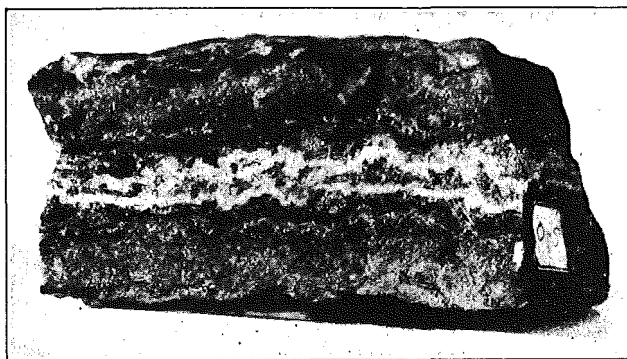
Plate V.—Quartz (dark) and adularia (white band) of the fifth stage of deposition, Oatman district.
