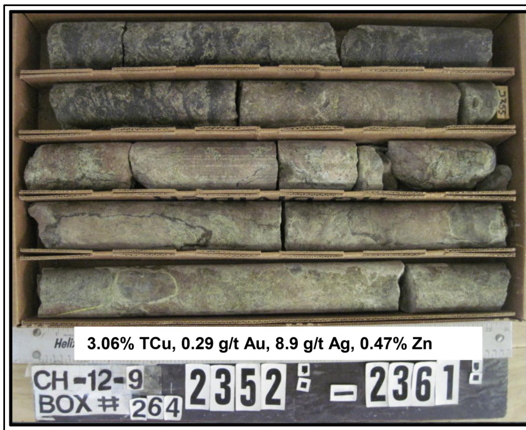
Figure 6. Magnetite-garnet-chalcopryite-sphalerite skarn in the Naco Limestone from east of the Joker Fault (photo from White and Thoman, 2014)
