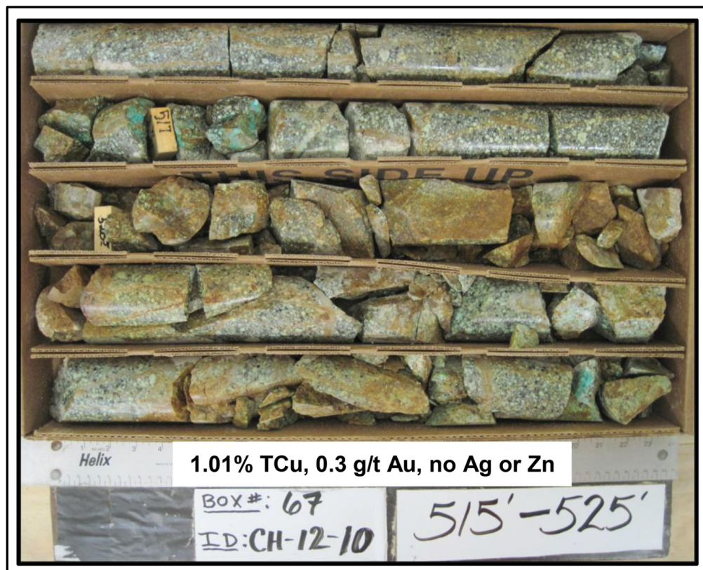
Figure 7. Oxide copper mineralization hosted by the Christmas Stock between the Christmas and Joker faults (photo from White and Thoman, 2014)
