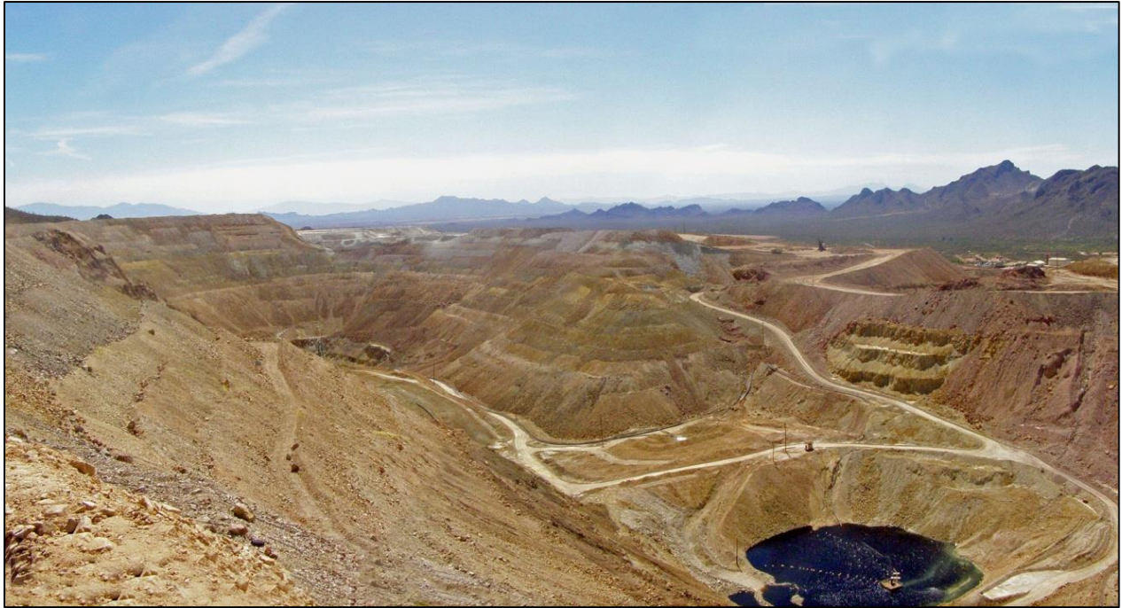
Figure 16. In-place leaching at the Oxide pit (looking southeast) (Photo taken in April 2016).
